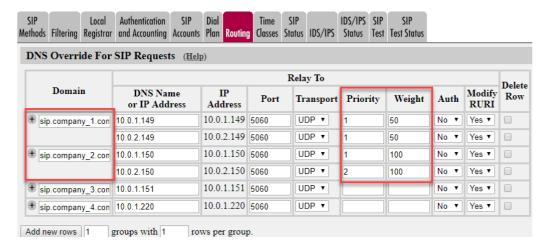
Here company\_1 will load balance between 10.0.1.149 and 10.0.2.149, while company\_2 will send all traffic to 10.0.1.150 and failover 10.0.2.150.
