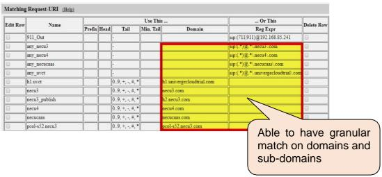
Based on the matching criteria, we used header manipulation while defining forward destinations as shown here:
