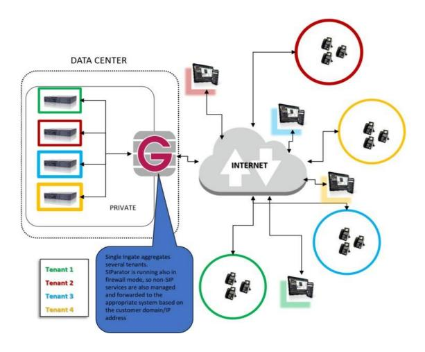
The diagram above shows the typical use case we are covering in this application note.
