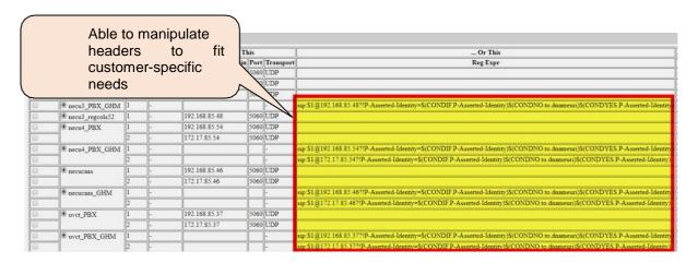
In this case for example a forward destination was defined as "necu4\_PBX\_GHM", and in that case the destination will be 192.168.85.54 with fail over 172.17.85.54, and
